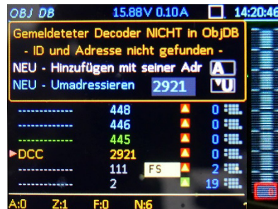
In this case: an unknown decoder is reported; it can be accepted as "NEW" with its current address (also automatically) or with a manually changed address.
