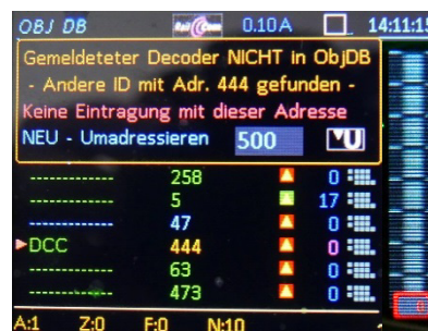
In this case: an unknown decoder is reported; however, its address is already assigned elsewhere in the database (therefore: ... no entry). A replacement address must be typed in, which can also be done automatically. Then the entry is made by forming a "NEW" line (left image).
