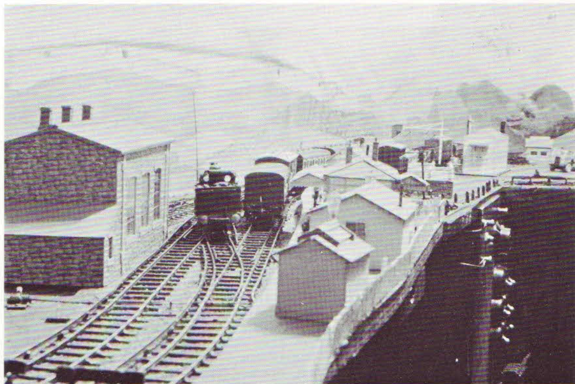
Outside third rail pickup on E F Colson's 1948 00 gauge GWR branch line layout. The control panel can be seen to the extreme right, incorporating an old-pattern miniature tumbler switch, once greatly favoured since it was easily available and, like most Woolworth's products of the period, cost only six old pence.
