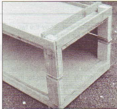
Close-up of the hinges of the folding baseboard. They are fixed to timber verticals which also form the corner pieces of the framing. A plywood facing has been added to the front and a ply capping has been securely glued to the top to provide a better fixing for the hinge screws. It is never a good idea to expect a screw in end grain to take any stress.
