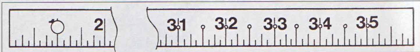
Drilling a yardstick to produce a simple trammel.
