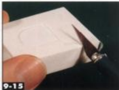
9-15 Corners must be glued tight, with no gaps. After the glue has dried, bevel the edges slightly with a hobby knife. Jeff Wilson
