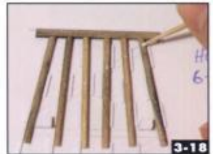
The sash drawing on the jig is a handy reference for adding glue before adding the sash. Jeff Wilson
