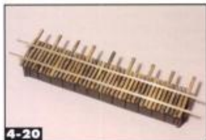
4-20 The long ties will support a walkway at the side of the bridge. The rails are glued in place with super glue. Jeff Wilson
