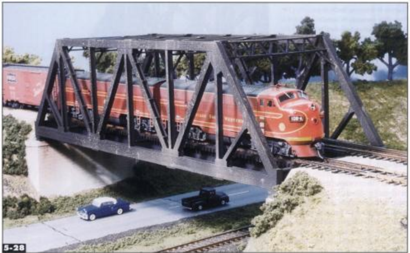
Walthers offers a kit for a double-track Warren truss in both HO scale (shown) and N scale. Jeff Wilson
