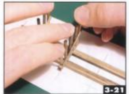
Mark the bent location on the bottoms of the stringers, apply a drop of white glue, and press the bent in place. Jeff Wilson
