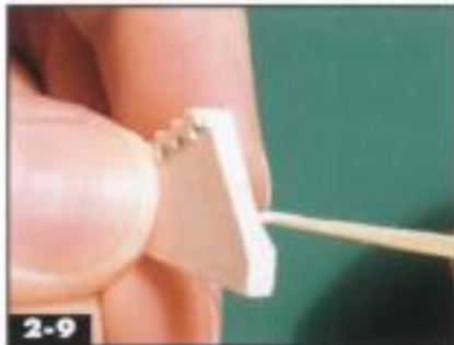
2-9 To fix a broken piece, apply a thin coat of white glue to one of the broken edges, then press the halves together firmly. Jeff Wilson
