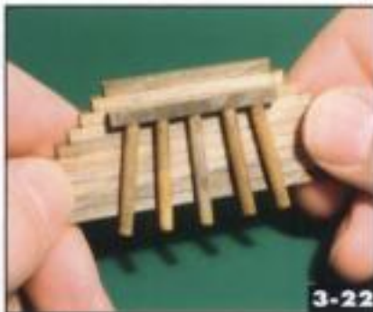
Glue the pile/cap assembly to the wood wall, making sure the distance from the top of the cap to the top of the wall is correct. Jeff Wilson
