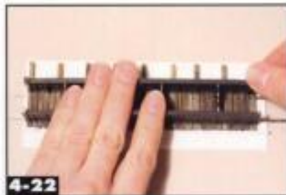
4-22 Run a bead of super glue along the bottom of each rail, then press the bridge in place. Hold it firmly for a few seconds until the glue takes hold. Jeff Wilson
