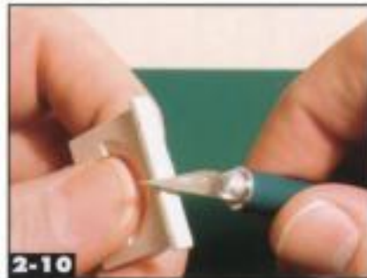
2-10 Use a hobby knife to remove flash and other stray material from plaster and plastic parts. Jeff Wilson
