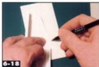
Trace the outline of the abutment onto a piece of .060" styrene sheet to make the trim pieces. Jeff Wilson
