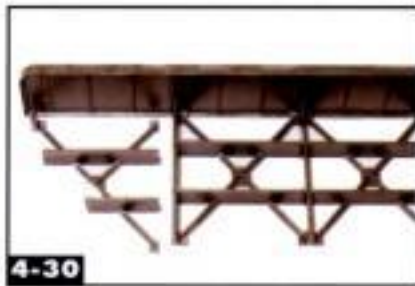
4-30 Cut an end from the spare floor section as shown at left, then glue it in place to the girder and main floor/beam section. Jeff Wilson
