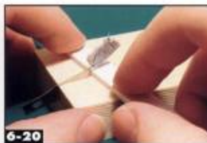
Pull strip plastic across a knife blade to bevel the edges. For safety's sake, make sure the blade tip is covered. Jeff Wilson
