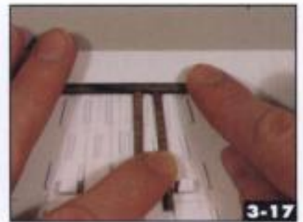
The jig holds the posts in line as the glued end is pushed against the cap. Jeff Wilson
