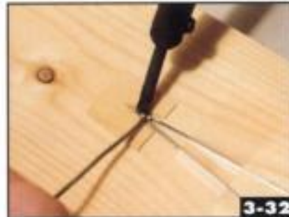
A Vgroove cut into a thin wood piece, glued to a larger board, holds the rails in place for soldering. Jeff Wilson
