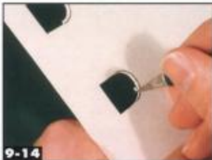
9-14 Draw the arch pattern on the styrene, then use a drill bit to start the curve. Carve out the rest of the curve with a sharp hobby knife. Jeff Wilson
