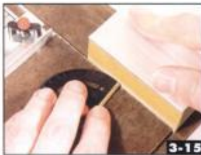
The NorthWest Short Line True Sander keeps parts aligned when truing the edges of strip and sheet material. Jeff Wilson
