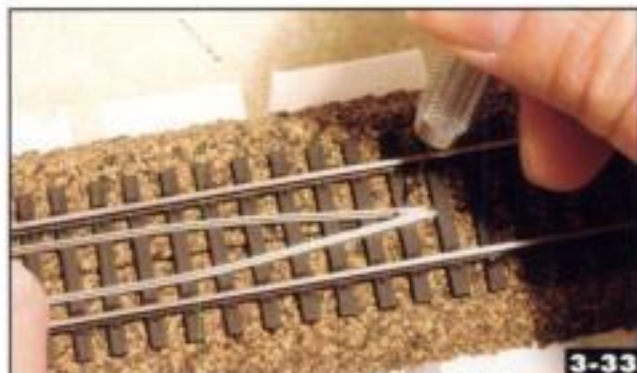
Position the frog and drill holes for the spikes that will hold it in place. Jeff Wilson
