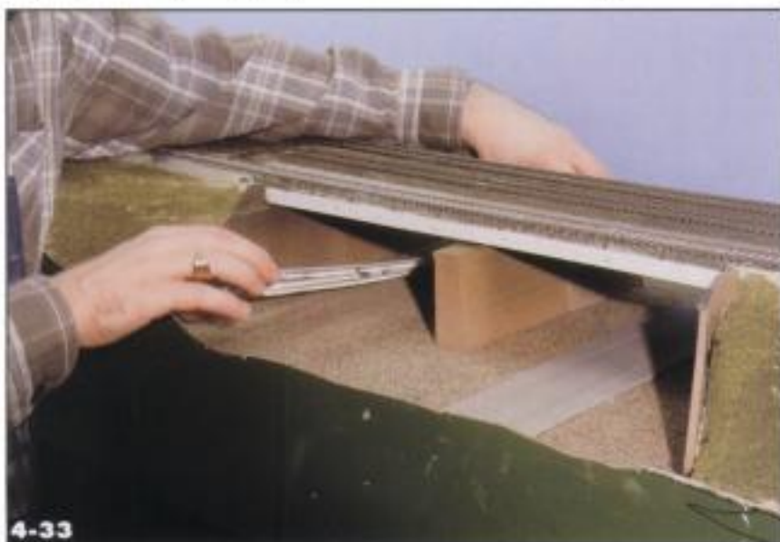
Model Railroader associate editor Cody Grivno modeled a girder bridge by first tacking sheet styrene to the edges of the plywood subroadbed, providing a smooth, easily glued surface for the girders. Cody Grivno
