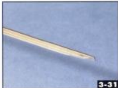
For the other side of the guardrail frog, bevel the end of another length of scrap rail to a mirror image of the first. Jeff Wilson
