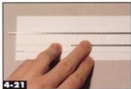
4-21 This styrene jig holds the rails in gauge upside down. The larger pieces of plastic at lower left and lower right align the edges of the ties. Jeff Wilson
