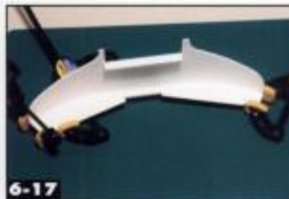
▼ To get the shape you want, clamp the contour pieces in position until the glue dries. Jeff Wilson
