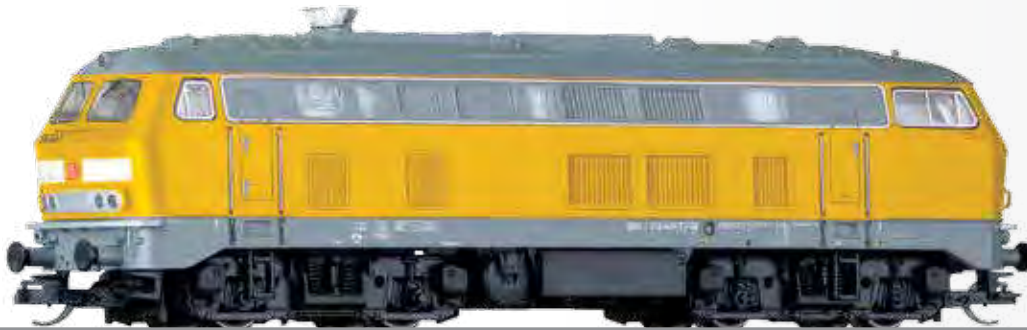
Diesellokomotive BR 218 der DB AG Diesel locomotive class 218 of the DB AG
