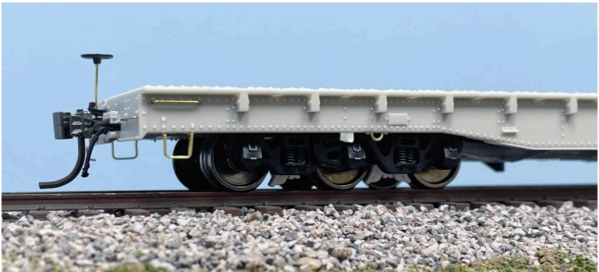
Wire grabs, buckeye trucks, simulated wood deck - this early pre-production flatcar has it all!
