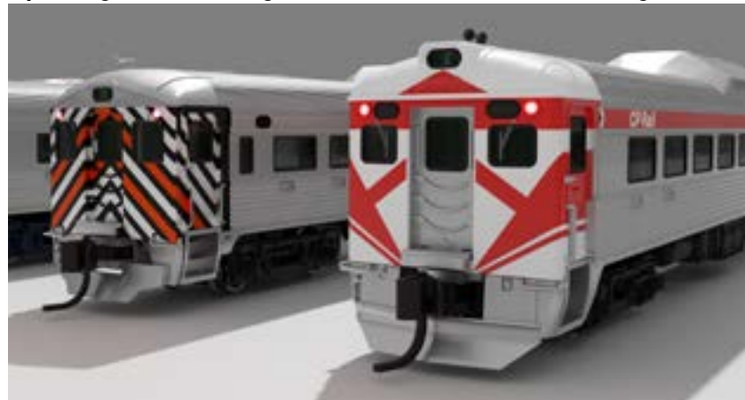
Operating Red Marker Lights on Phase 1 (left) and Phase 2 (right)
