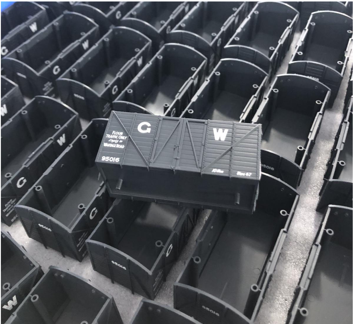
The GWR Mink A (V14 & V16) vans have had their lettering applied and will shortly be entering the assembly stages
