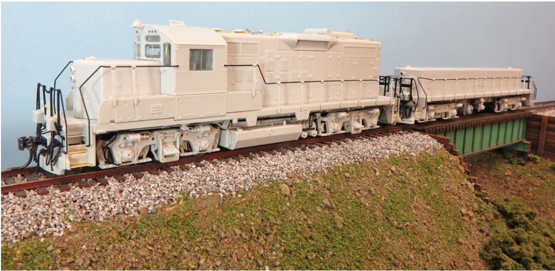
Note the strobes and extra details on the GP9RM slug mother . Preproduction samples subject to revision.
