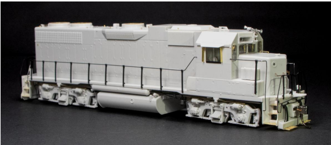
The PC and CR GP38s have the correct two-strap cab signal box. Preproduction samples subject to revision. (Production models will not have a crooked horn!)
