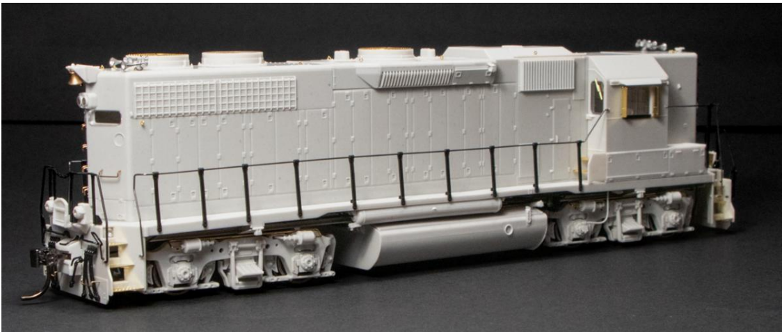
Note the walkway lights on the side of the hood of the NS GP38 . Preproduction samples subject to revision.
