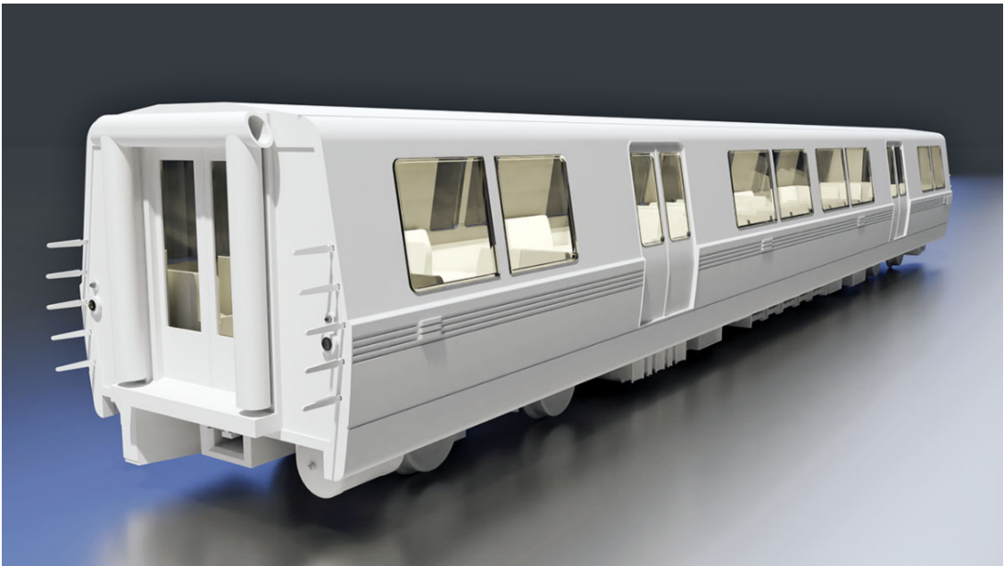
This is an unpowered "B" car. 3D renders are subject to revision.
