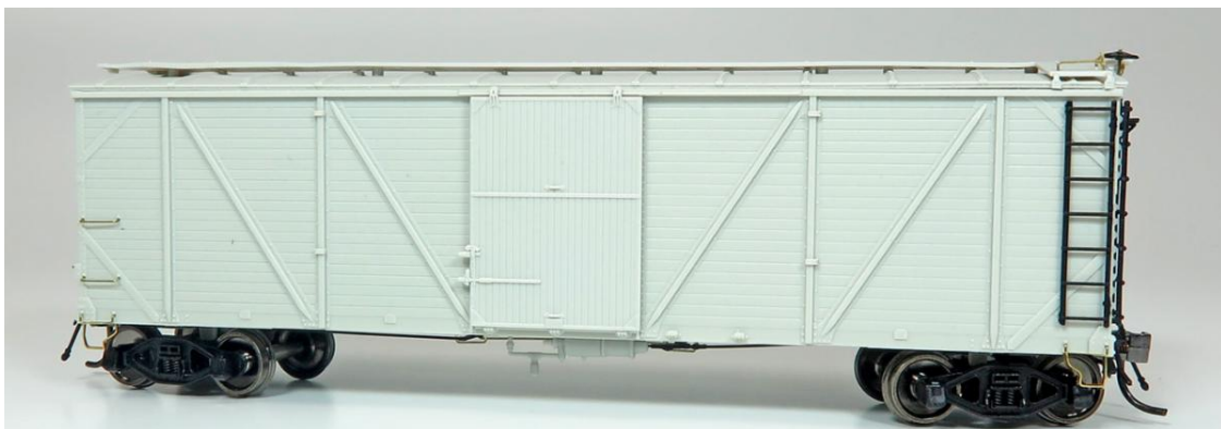
This is a B-50-15 with Murphy Radial roof and wood sides. Note the K brakes. Pre-production samples are subject to revision.
