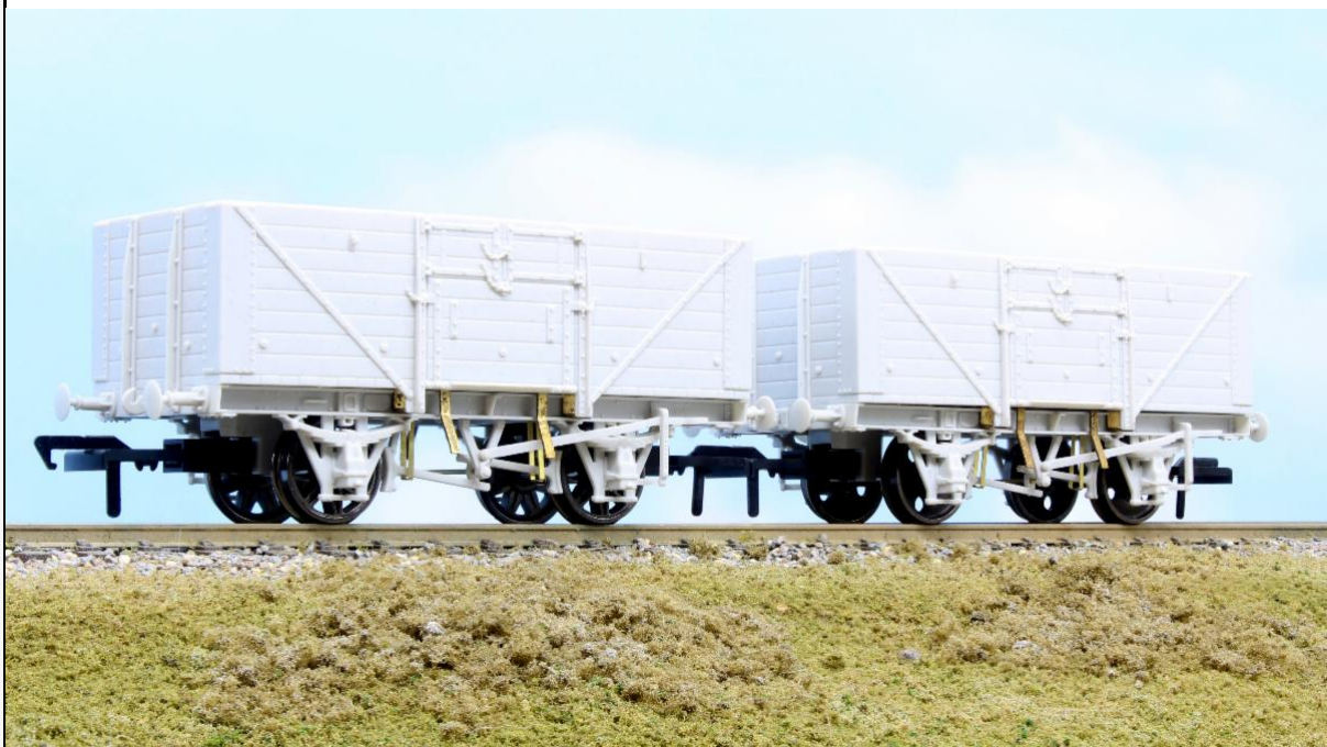
So what's the difference between these EPs? Well, they are both Dia. 1379s fitted with Morton brakes and, as you can see, there are split-spoke and disc wheels variants.
