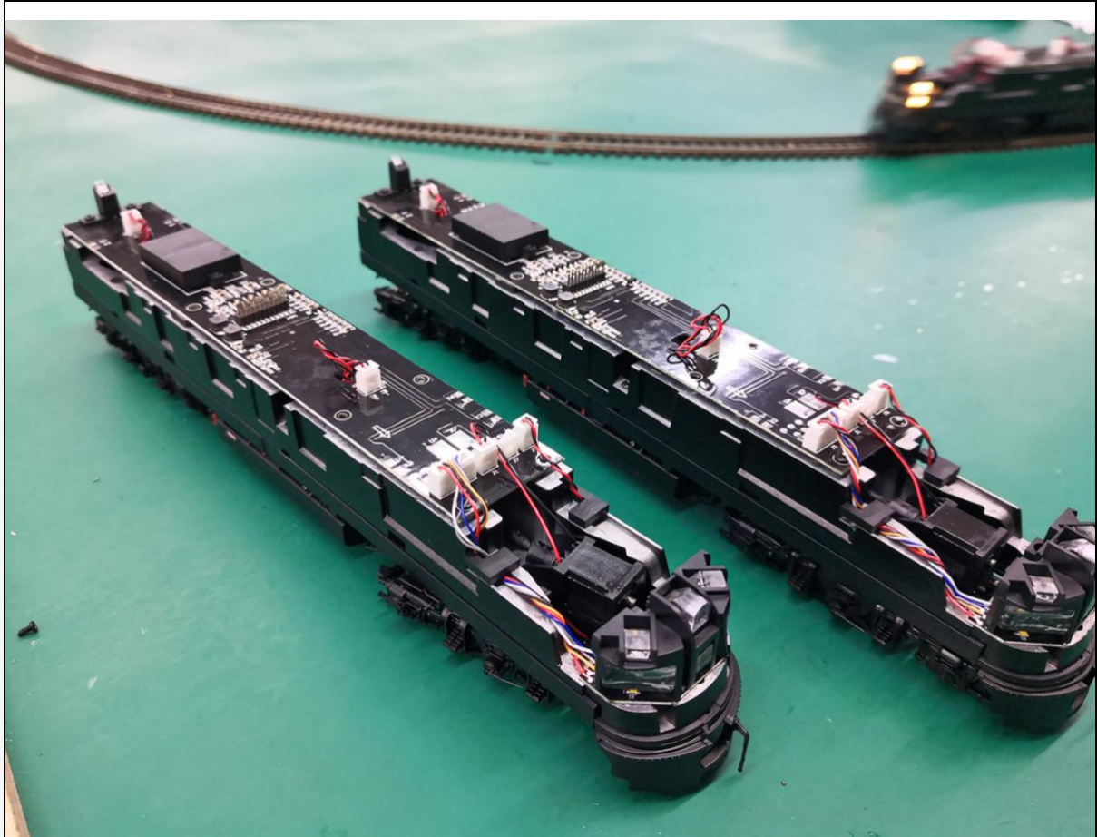
HO Scale E8 chassis, all ready for the bodies. These are the Amtrak anniversary units.
