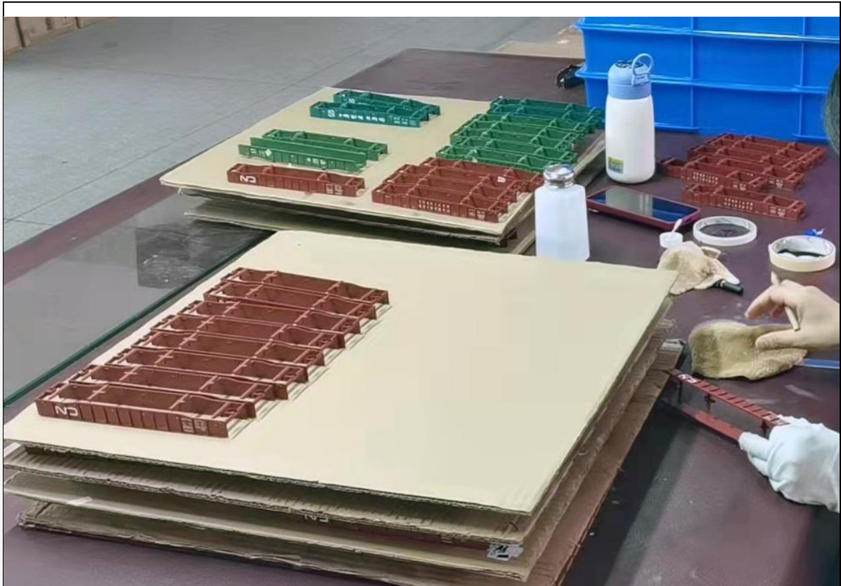
A handful of HO Scale 52' Mill Gondolas await to have their floors attached.
