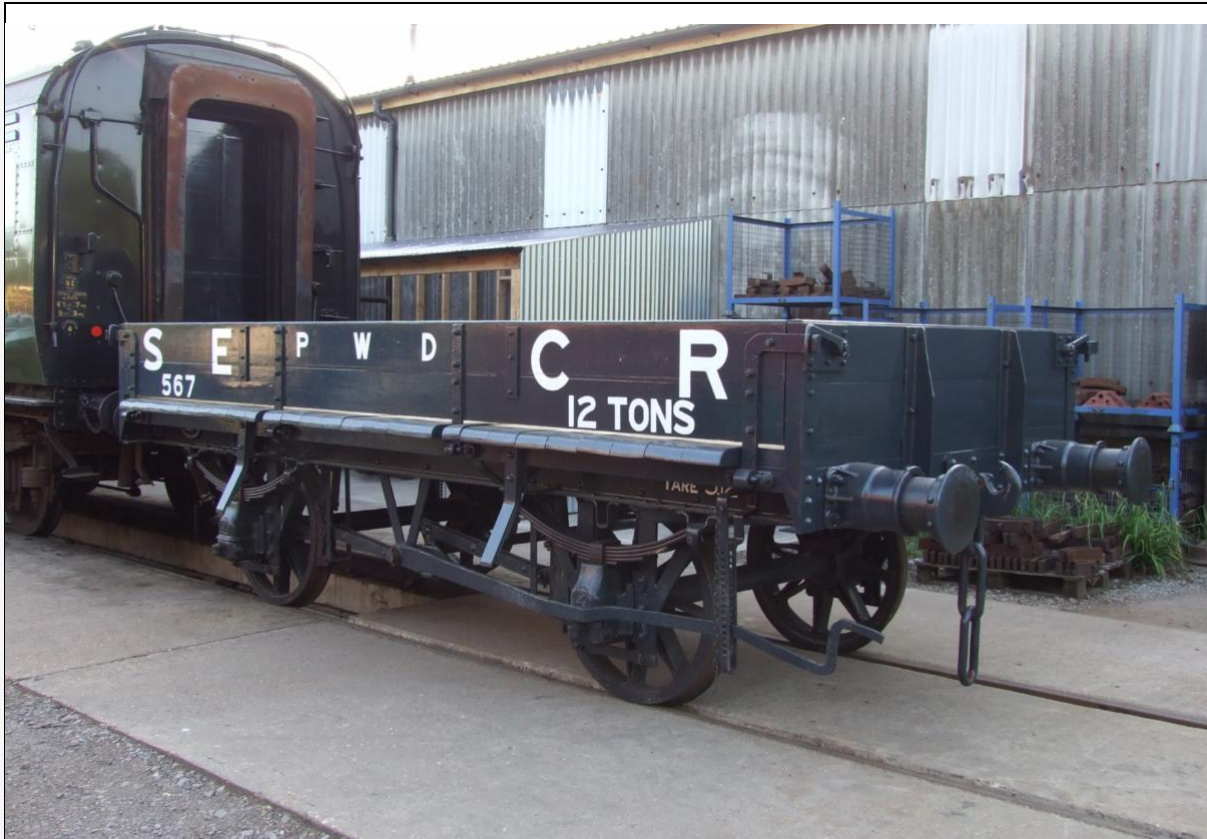
Replica SECR Dia. 1744 two-plank ballast wagon No. 567 looks splendid after completion in 2012.
