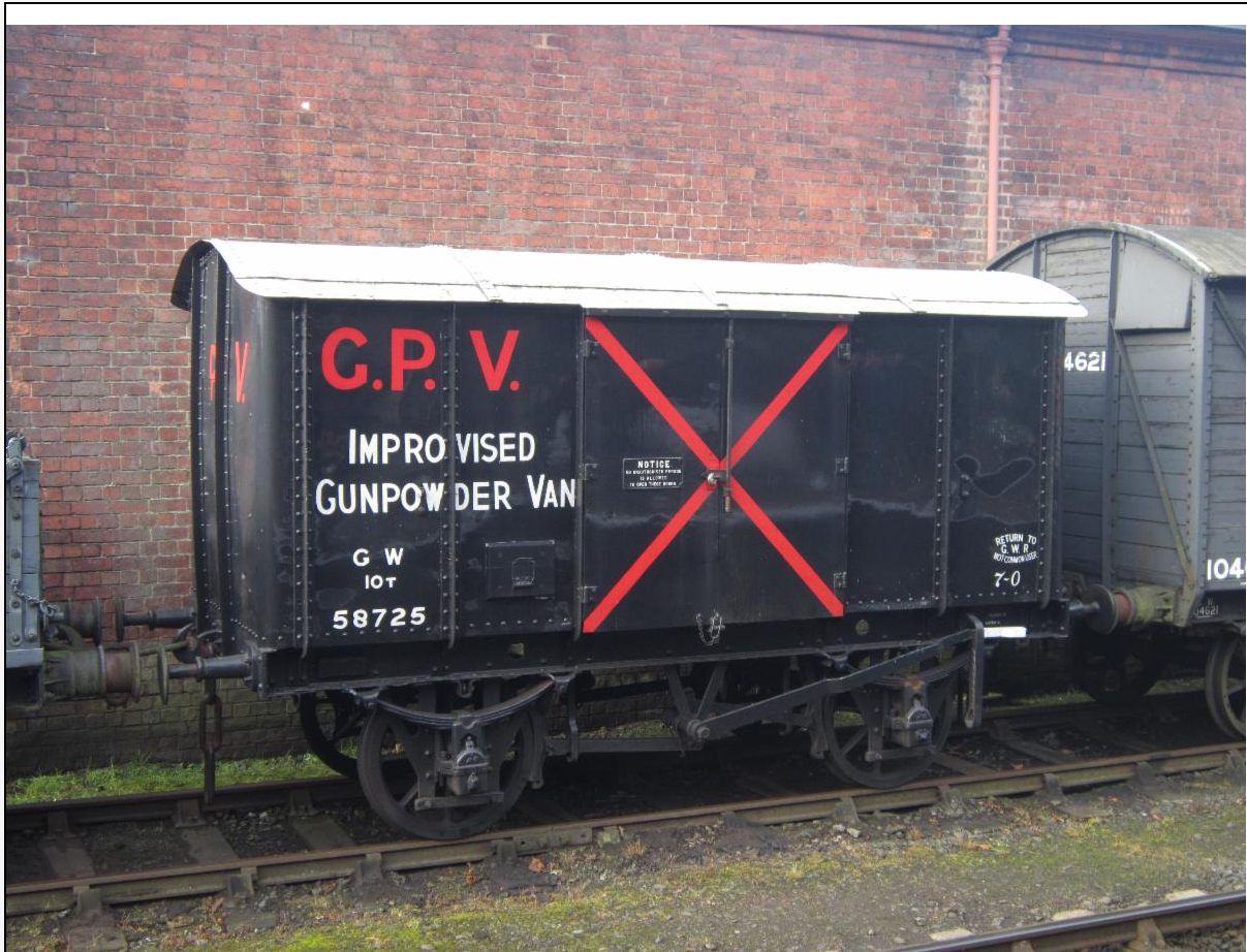
Their metal construction made the 'Iron Minks' ideal gunpowder vans during times of war. No. 58725 was turned into a GPV in 1938 and loaned to the Southern Railway. It's now based on the Severn Valley Railway . Photograph: G Price
