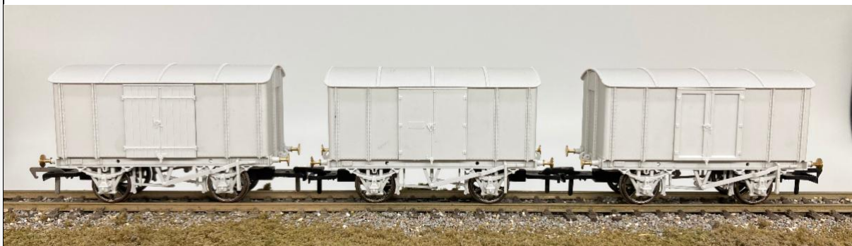
Here, you can see the three types of door we've tooled: replacement wood, those fitted to gunpowder van conversions and the original design.
