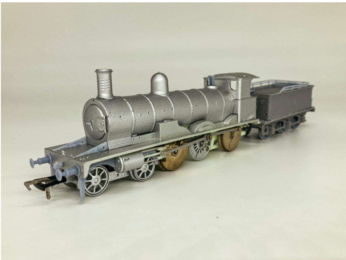
This working 3D printed sample has enabled us to prove that the frames around the bogie won't impair running through trainset curves.
