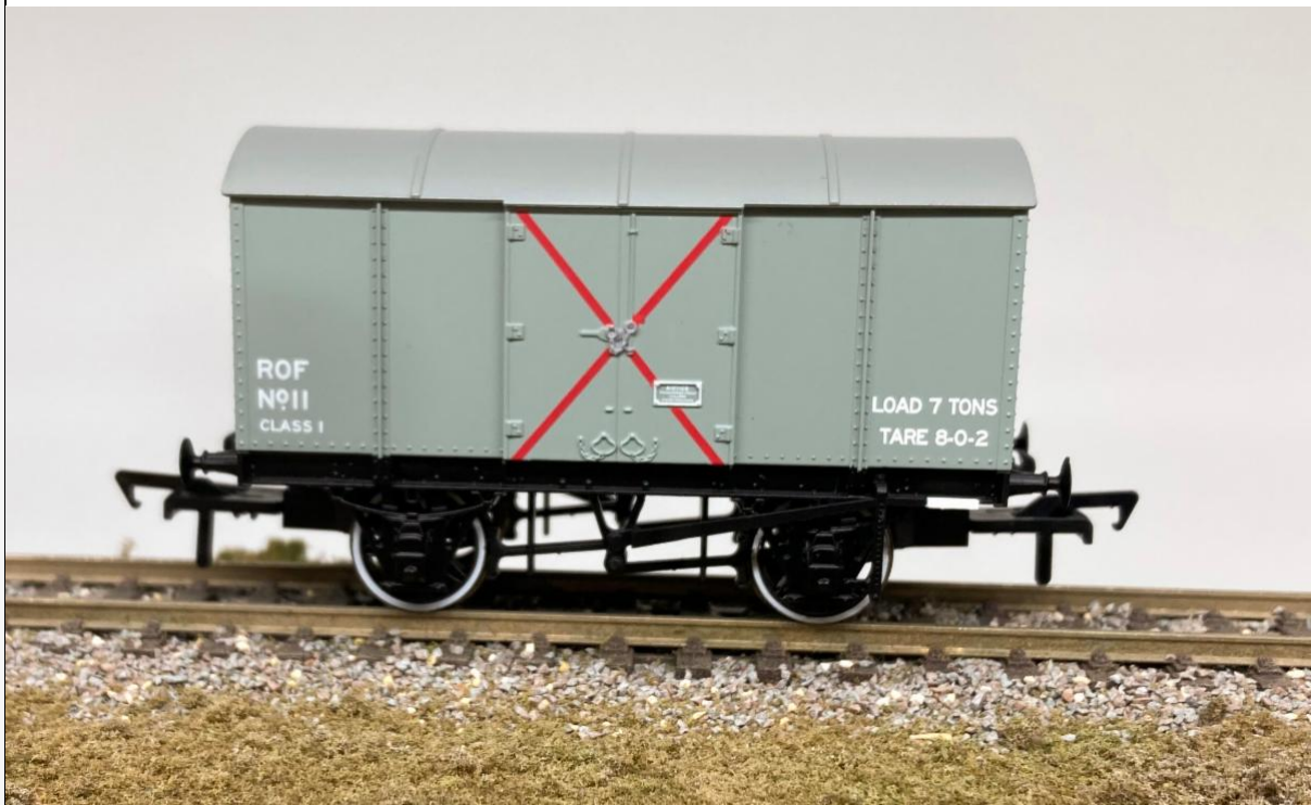
And here is an RCH pattern GPV carrying Royal Ordnance Factory grey (902011). If you want to see more GPVs, there are more towards the end of the newsletter. But don't look just yet in case you miss out on more cool stuff!
