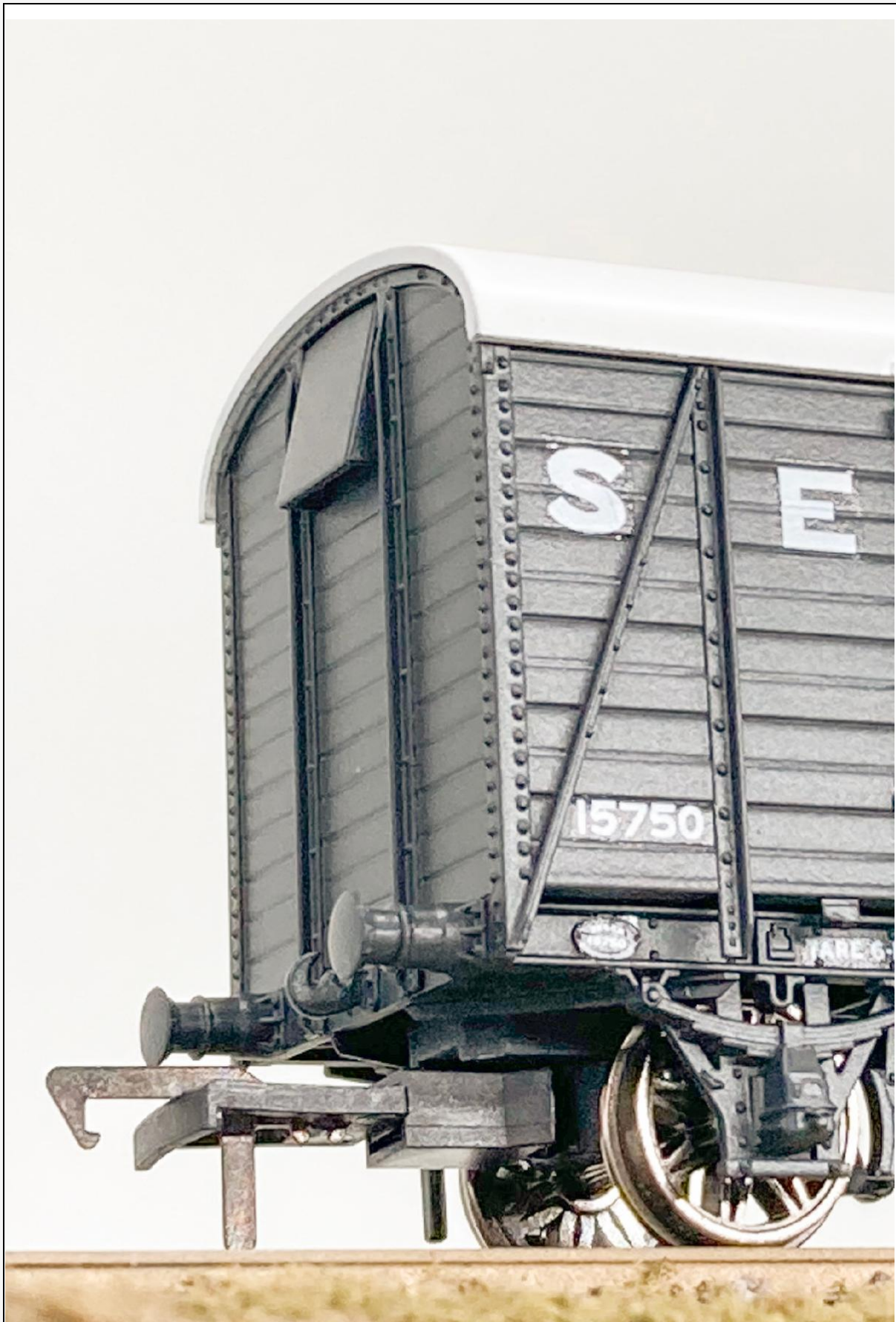
Is this a first in British-outline ready-to-run 'OO'? The separately-fitted vents means that you see the distinctive 'hole' underneath them.
