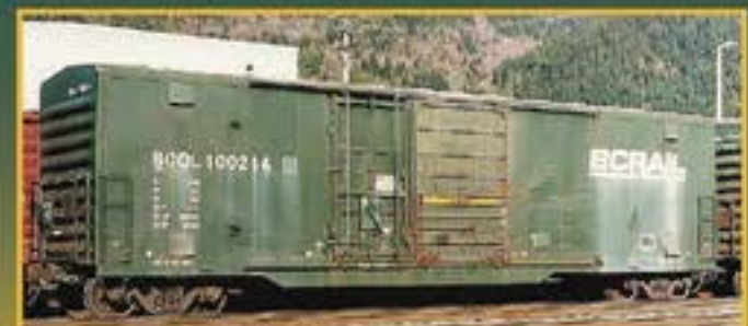
BCOL - 100,000 series, re-built 1990 w/vents
