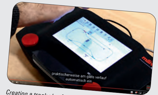
Creating a track plan for an H0 model railroad – Instructions for the Märklin CS3
