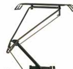
Pantographs can be raised and lowered by a motor
