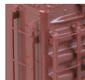
Scale ladders and grab irons.
