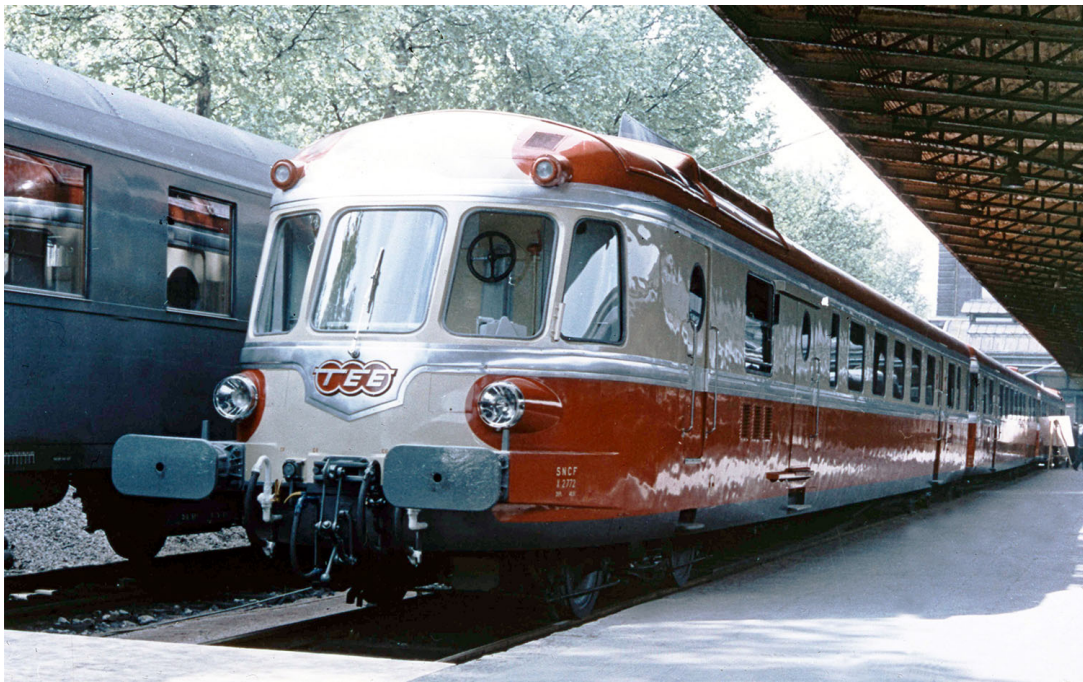
SNCF, diesel railcar RGP I with trailer, red/beige TEE livery, ep. III
