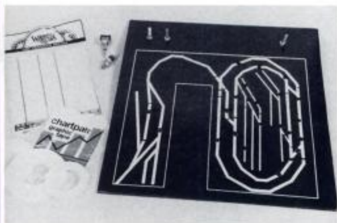
transfer lettering from Woodland Scenics provide all the materials you need to decorate the control panel. Cut the Chartpak tape with a sharp hobby knife. Be sure the panel is completely dry before applying the tape and lettering, or you may leave fingerprints in the surface.
