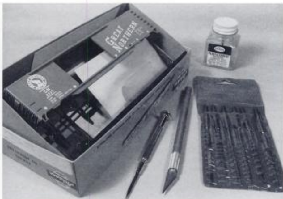
Assembling car kits is not difficult—most can be completed in five minutes to half an hour. Glue, a hobby knife, a small screwdriver, and a file set are all that's usually needed to assemble freight car kits.
