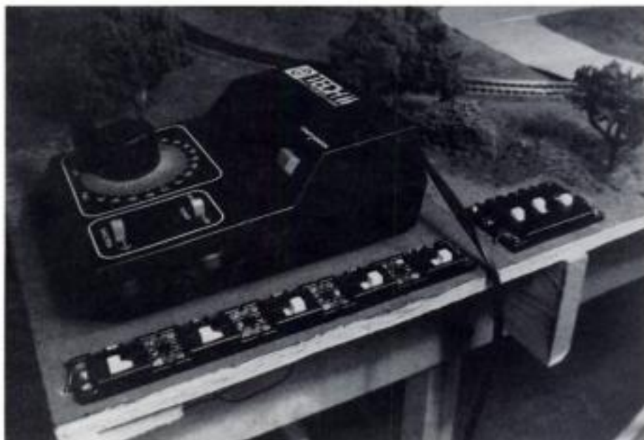
The control panel grows in this stage, too, with the addition of the control switches for the blocks and the remote control turnouts. Remove just enough ground covering to make room for the new switches.
