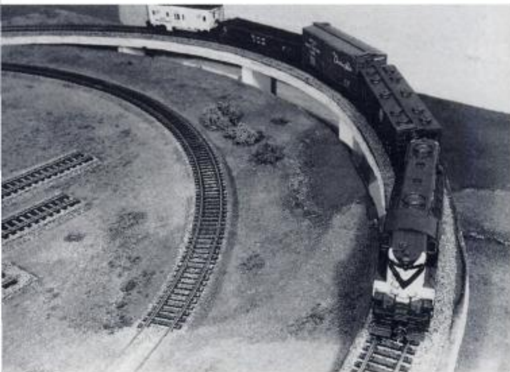
Raising the track at one end of the layout left a hole underneath. Simple hardshell scenery plugs the hole and makes a realistic track embankment.
