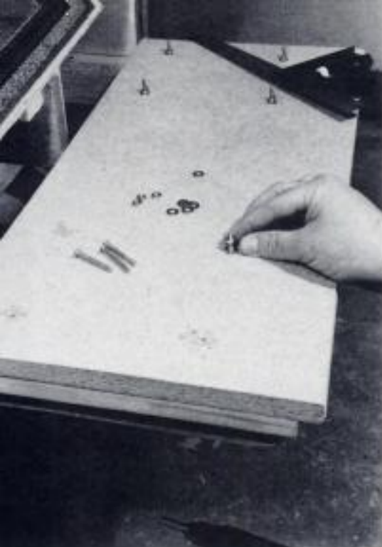
LEFT: The MRC power packs on the CC rest in place on the control panel on top of screws. The power pack instruction sheets contain the dimensions that show the exact location of the screws. This method secures the packs, but it also allows you to remove the packs from the panel, should the need arise. ABOVE: This view shows the finished control panel with the selectors and switch controllers installed. This panel provides more work space and places the operator right in front of the yard for a better view of the action.
