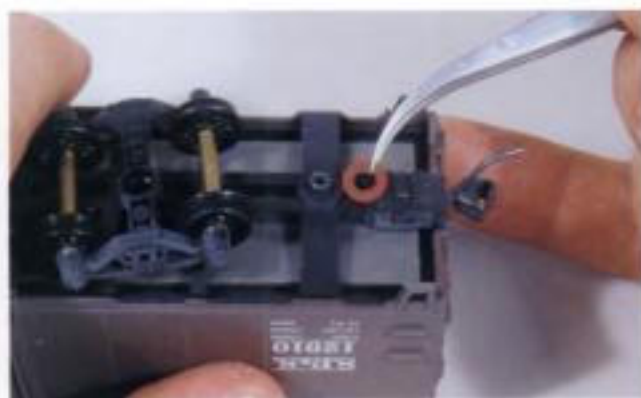
Fig. 3-14. A slightly low coupler can be corrected by adding a thin shim washer between the car bolster and truck, as on this Athearn boxcar.
