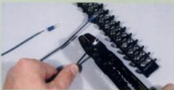
Fig. 3. Add spade terminals by threading them onto the stripped end and crimping them in place.
