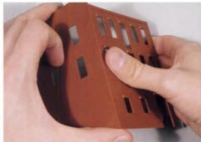
Fig. 11-2. Test-fit the corners to make sure they fit snugly against each other. This structure includes an extra lip on the rear of one wall to help locate the neighboring wall.
