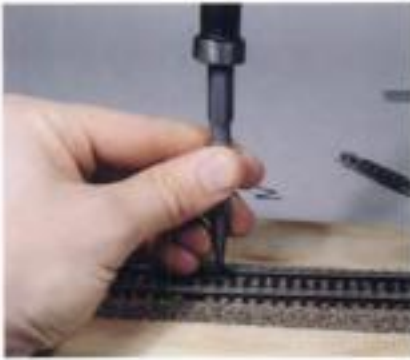
Fig. 9-9. Use a nail set to drive track nails below rail level.
