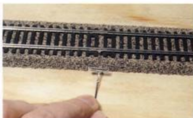
Fig. 9-12. Terminal rail joiners are easy to use, and they will be nearly invisible when the track is ballasted.
