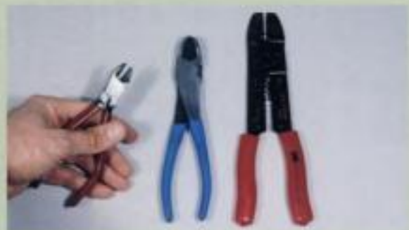
Fig. 2. Small (6") and large (8") wire cutters and a stripper/crimper are vital for working with wire.
