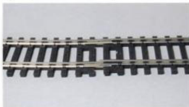
Fig. 9-6. A common mistake is to allow one rail to slide up and over a rail joiner. Pull the track apart and reconnect it properly.
