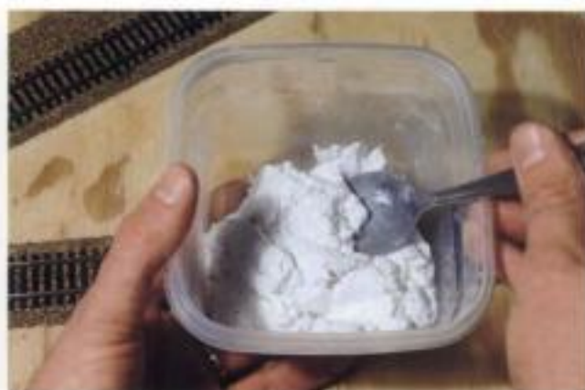
Fig. 12-4. Add water gradually and mix thoroughly until the Sculptamold reaches a fairly thick consistency like this. It shouldn't be runny.
