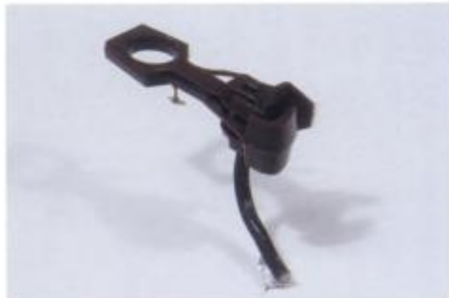
Fig. 3-5. Life-Like's Proto 2000 coupler is molded in plastic, with built-in springs on the side of the shank.
