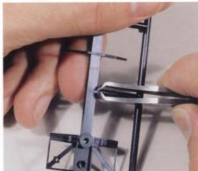
Fig. 2-10. Flush sprue cutters are designed to trim parts cleanly.
