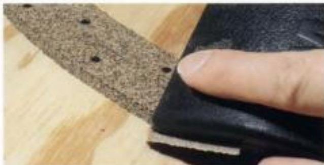
Fig. 8-8. Use a sanding block with 120-grit sandpaper to remove the burr at the top of the bevel on the cork.
