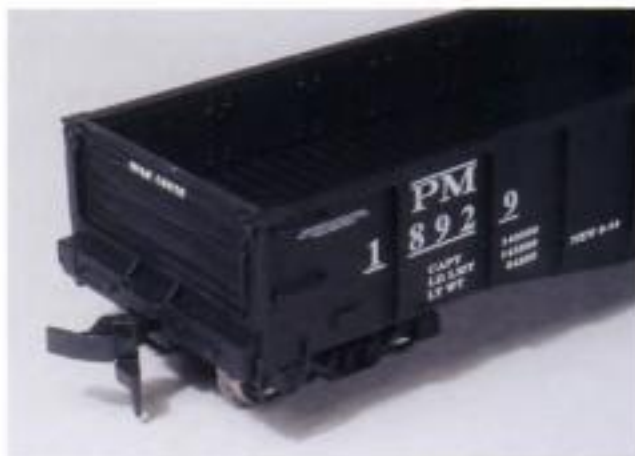
Fig. 3-1. Horn-hook couplers were once the industry standard, and they still come as standard equipment on some new cars.
