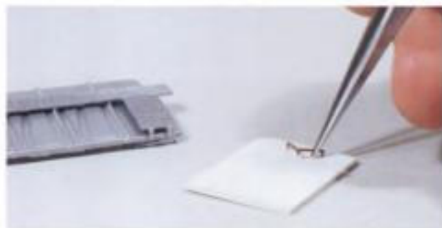
Fig. 6-13. If a detail part has mounting pegs, dip the pegs in cyanoacrylate, then set them in place on the model.
