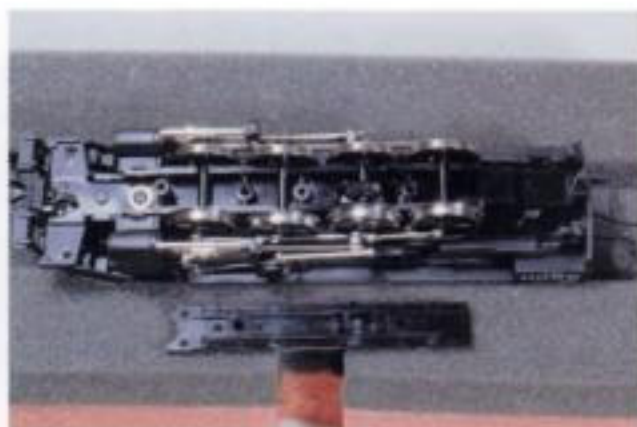
Fig. 5-7. Removing the bottom plate provides access to the axle bearings as well as the driver gear.
