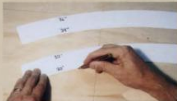
Fig. 3. These templates, made from styrene, hardboard, or thin plywood, are handy for drawing broad curves.
