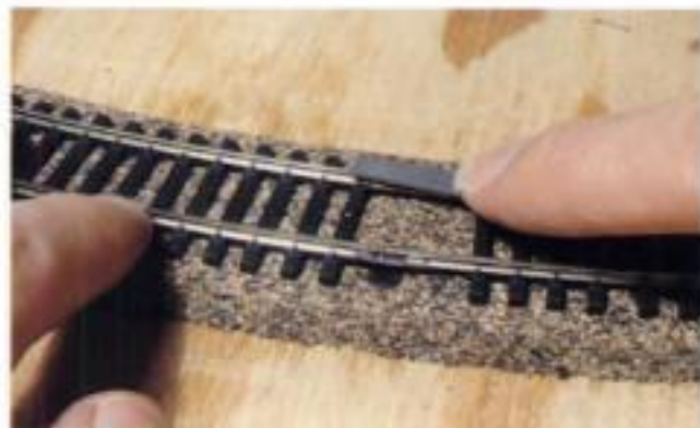
Fig. 9-20. Give the railhead a couple of passes with a needle file to make sure the joint is smooth.
