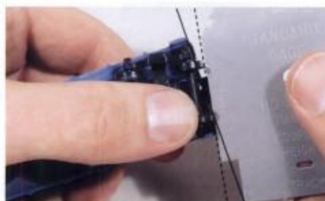
Fig. 4-2. The flanges should rest in the notches on the NMRA gauge. This wheelset is narrow in gauge, and the flanges are deeper than NMRA recommends.
