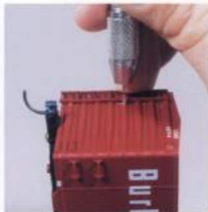
Fig. 6-16. Some cars require mounting holes to be drilled for details on the ends or sides.
