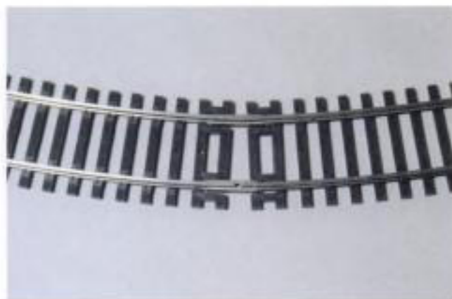
Fig. 9-7. Forcing tracks into a too-tight curve creates a sharp angle and a gapped rail, which will often lead to derailments.
