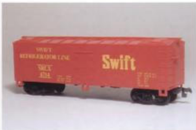
Fig. 1-7. The Life-Like train set cars have molded-on detail and snap-on trucks with truck-mounted couplers.
