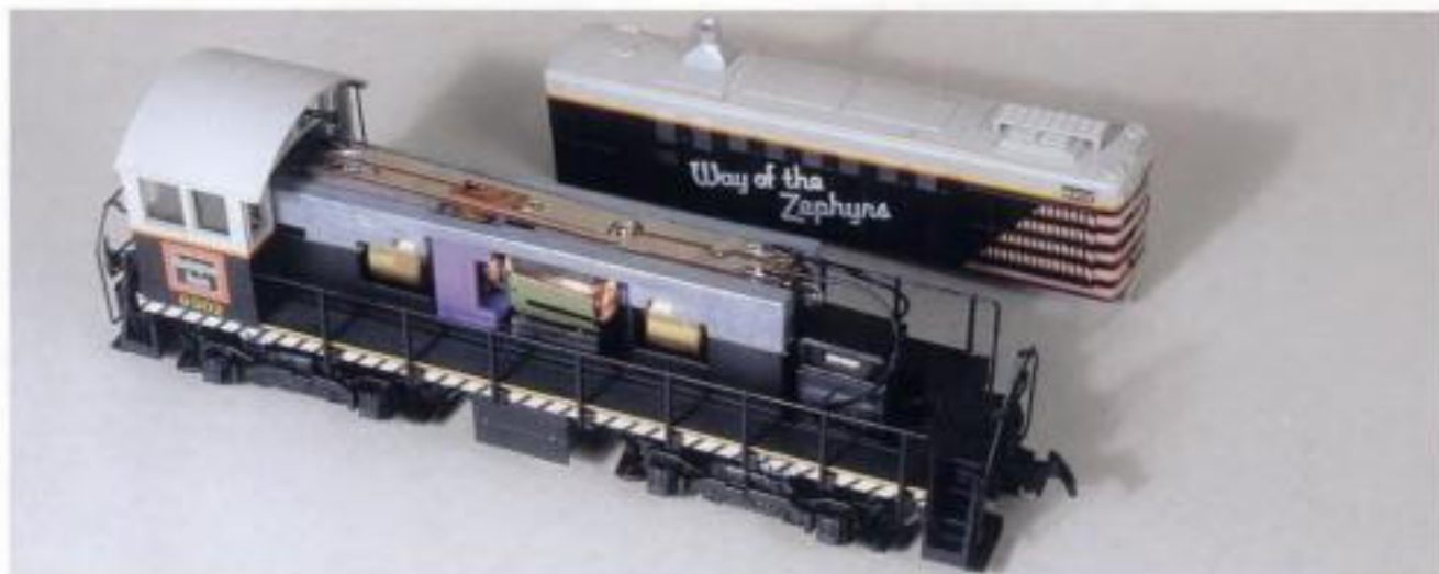
Fig. 1-4. This Atlas engine is a high-quality, realistic model with all axles powered.
