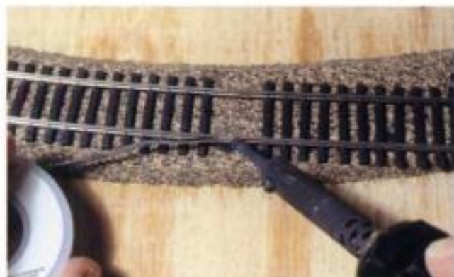
Fig. 9-18. Make sure the joint is tight and square, then solder the rails at each joint.
