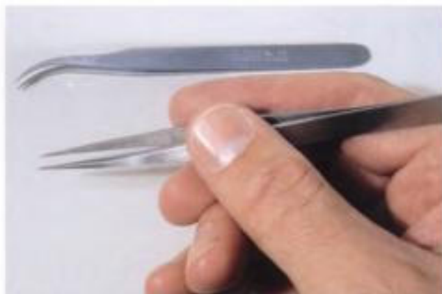
Fig. 2-5. Make sure tweezers have sharp points that match each other well.
