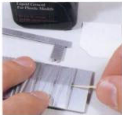
Fig. 6-11. Use glue sparingly, as on this running board support.
