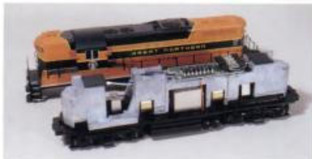
Fig. 5-1. This Proto 2000 GP9 shows typical diesel model construction. Lifting off the injection-molded styrene shell reveals weights covering the engine and mechanism and all wiring routed through a circuit board mounted at the top.
