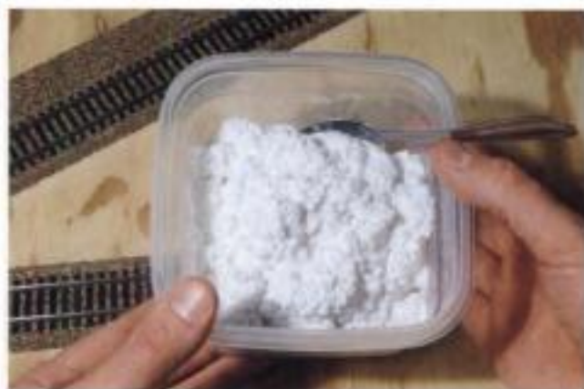
Fig. 12-3. Dry Sculptamold resembles plaster, but with more fiber content.
