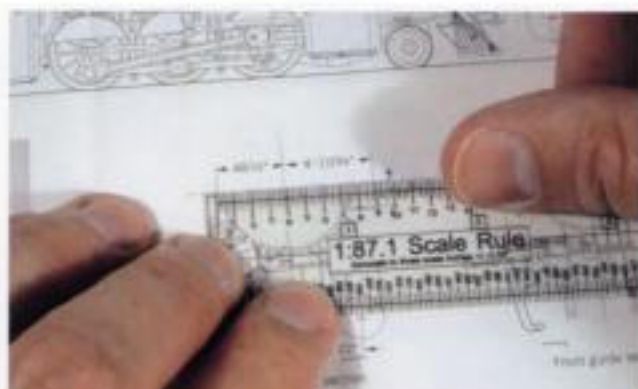
Fig. 2-4. See-through rules, like this one from Scale Card, are handy for measuring drawings and models.
