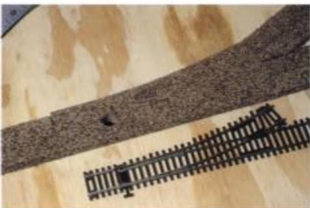
Fig. 9-28. If you plan to use under-table switch machines, drill a \frac{1}{8} " hole through the table and roadbed under the center of the turnout throw bar before laying track.
