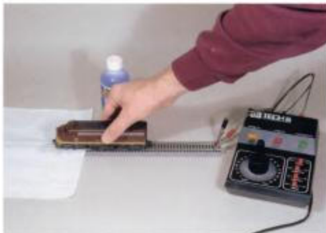
Fig. 5-8. Place cleaning fluid on a paper towel across the tracks. Running the engine over the towel cleans the wheels quite effectively.
