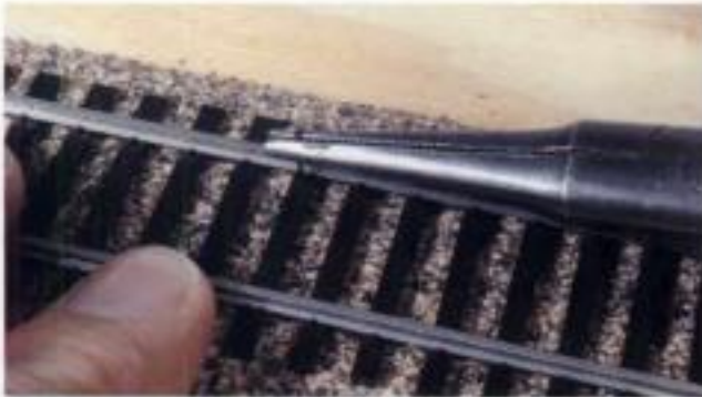
Fig. 9-11. Insert spikes into place next to the rail (above left), then use the side of the needle-nose jaws to press the spikes all the way into place (above right). The spikes provide a more realistic look than do track nails (below).
