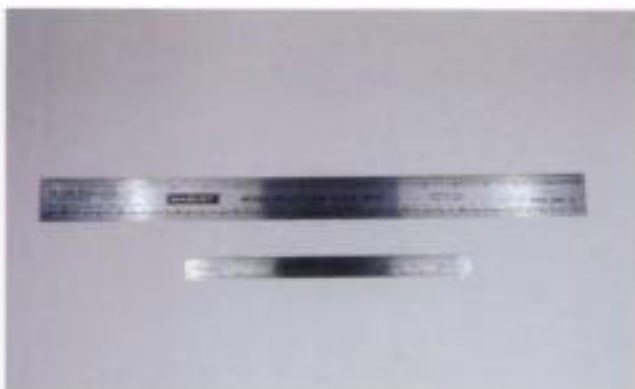
Fig. 2-3. A foot-long steel scale rule is among the most essential tools. A shorter rule with inch and millimeter markings is also handy.
