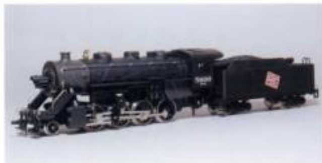
Fig. 5-5. This International Hobby Corp. 2-8-0 has an injection-molded styrene shell that is attached to the frame by means of a screw and plastic tabs.
