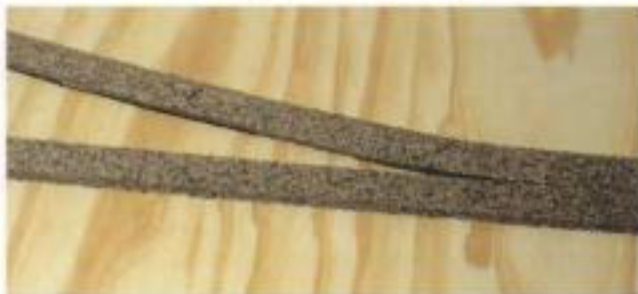
Fig. 8-6. When fabricating a turnout pad, start with the outside pieces.
