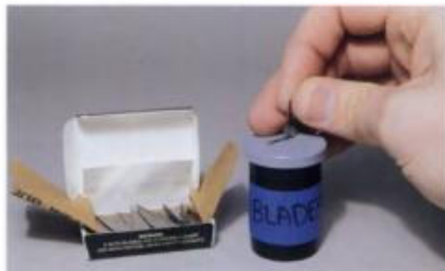
Fig. 2-2. Bulk packs (such as this box of 100 X-Acto no. 11 blades) are economical. Place old blades in a sealed plastic container.
