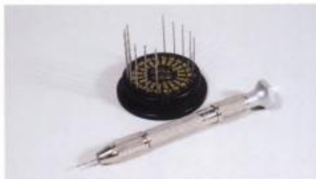
Fig. 2-9. A pin vise is a handy tool for drilling holes with small (nos. 61 to 80) bits.
