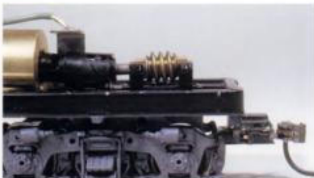
Fig. 5-3. Removing the cover atop the truck tower provides access to the worm and top of the truck gears.
