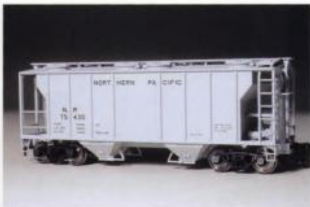
Fig. 1-6. The Atlas cars, from the firm's standard line, have excellent detailing, metal wheels, and body-mounted couplers.
