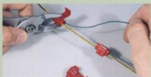
Fig. 4. Suitcase connectors: use a channel lock to push the metal strip in place, then close the cover.
