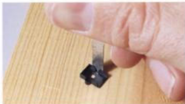
Fig. 3-20. Cut off the side mounting pods on the Kadee coupler box before mounting it.
