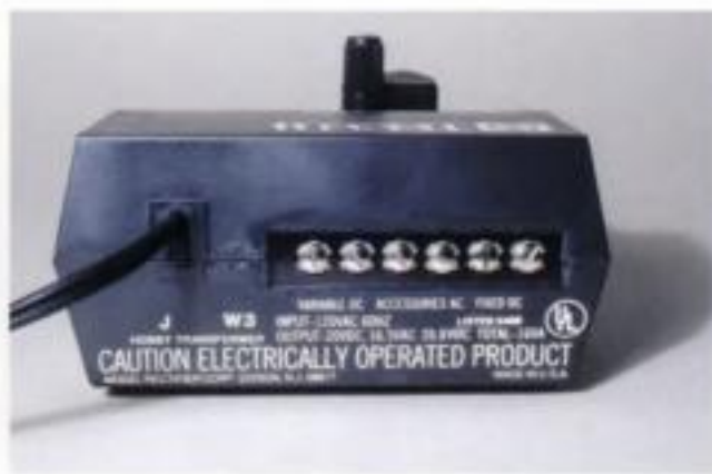
Fig. 10-2. All packs have a variable DC output for trains; most have an AC output for accessories, and some have an additional fixed DC output for accessories.
