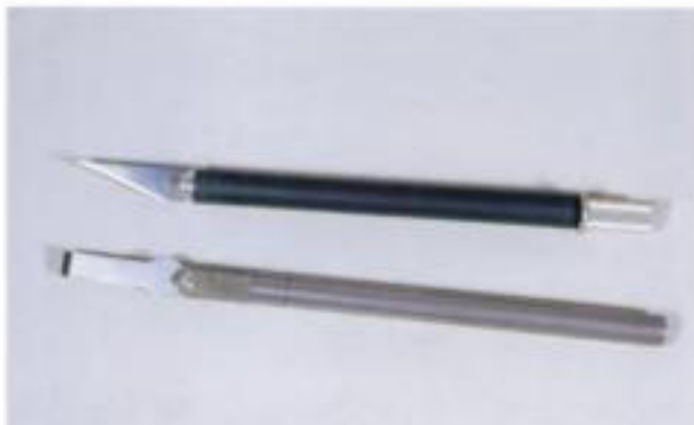
Fig. 2-1. Knives with no. 11 (top) and no. 17 (bottom) blades are both handy.
