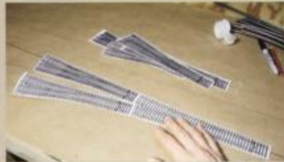
Fig. 4. While trimming turnouts to size, tape templates in place to prevent the track from becoming misaligned.
