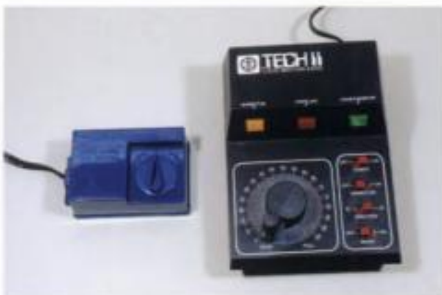
Fig. 10-1. Power packs reduce house current to low-voltage DC for trains. The pack at left is from a Life-Like train set; the MRC pack at right has many advanced features.
