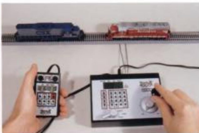
Fig. 10-7. The Digitrax Zephyr is a basic DCC system. Several hand-held throttles can be used at once to run multiple trains.
