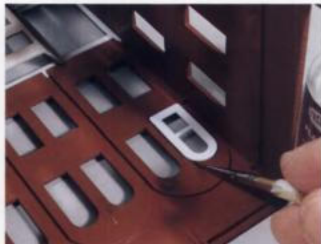
Fig. 11-8. Touching a brush of liquid cement to the window joint from behind lets capillary action pull the glue into the joint.
