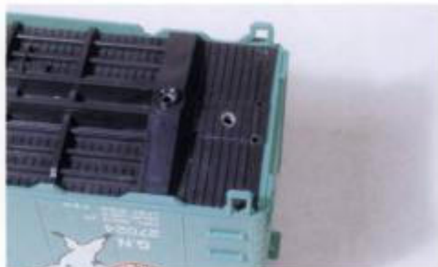
Fig. 3-19. To body-mount a coupler to a car, use the lid of the coupler box cover to mark the hole location, then drill a no. 50 hole and tap it 2-56.
