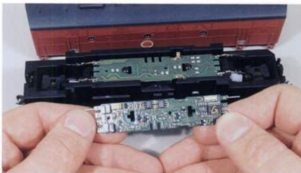
Fig. 10-10. Adding a decoder to this Stewart Hobbies F unit involved removing the original circuit board and screwing this new circuit-board-style decoder in place. The engine connection tabs and track wires had to be removed and then reinstalled.
