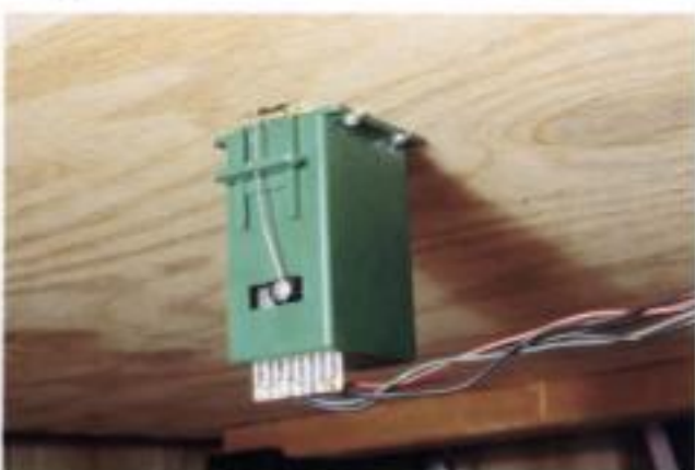
Fig. 9-26. Slow-motion machines like this under-table Tortoise use a motor to throw the control wire back and forth.
