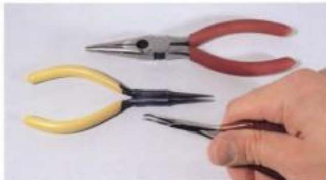
Fig. 2-7. Needle-nose pliers in different sizes are handy for grasping small parts.
