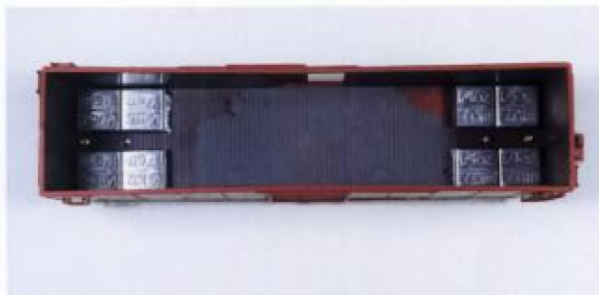
Fig. 6-18. Since the open doors make the middle of the interior visible, weights were added out of sight at each end. Be sure to balance the weights for stability.
