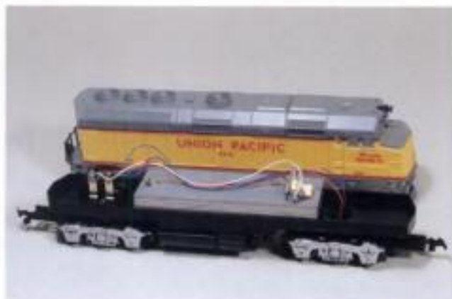
Fig. 1-5. The Life-Like train set engine has an inexpensive motor that powers only one truck. It also isn't as nicely detailed as the Atlas model.
