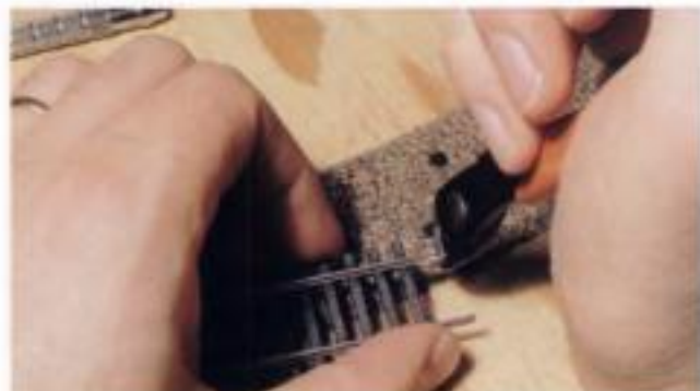
Fig. 9-17. Use rail nippers or a razor saw to cut the rail at the mark.
