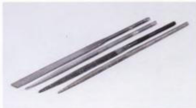
Fig. 2-6. Needle files (or jeweler's files) are available in many shapes.
