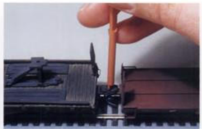
Fig. 3-11. Cars can be uncoupled using a small screwdriver or a tool such as the Accurail Switchman.
