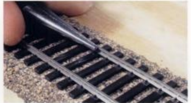
Fig. 9-11. Insert spikes into place next to the rail (above left), then use the side of the needle-nose jaws to press the spikes all the way into place (above right). The spikes provide a more realistic look than do track nails (below).
