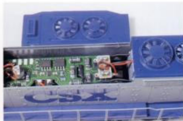
Fig. 10-8. This Atlas SD35 has a DCC decoder built into its circuit board. Moving the plug at right allows modelers to switch from DCC to standard DC control.
