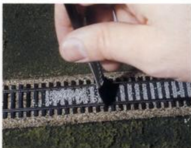
Fig. 12-18. Use a soft, flat brush to distribute the ballast evenly between the ties.
