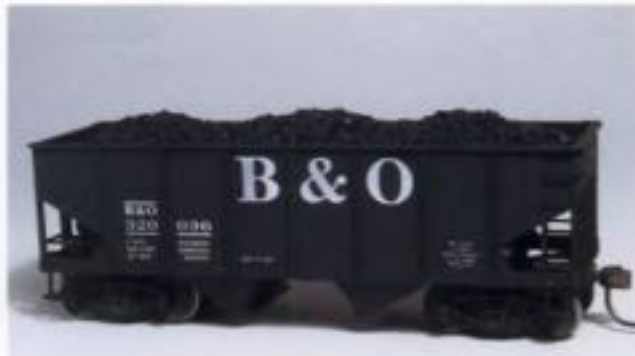
Fig. 6-24. Adding the load was a simple matter of sliding it in place. The car has also received a coat of chalk weathering.
