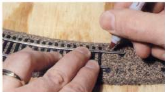
Fig. 9-16. Flex the end of the track into position, then mark the long rail at the point where it is even with the other rail end.
