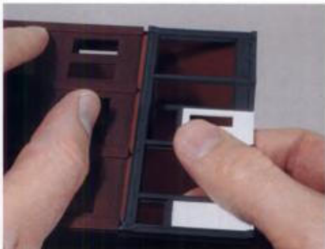
Fig. 11-7. Glue the subassemblies together. Make sure there's no paint on mating surfaces.
