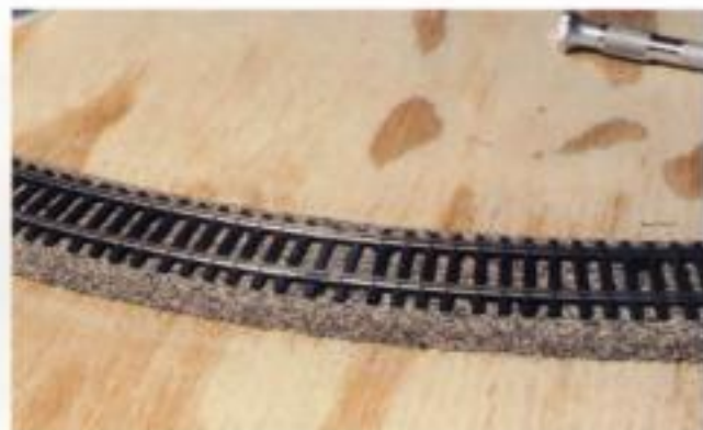
Fig. 9-21. Finish the joint by filling the gap with a couple of ties under the rail joiners.
