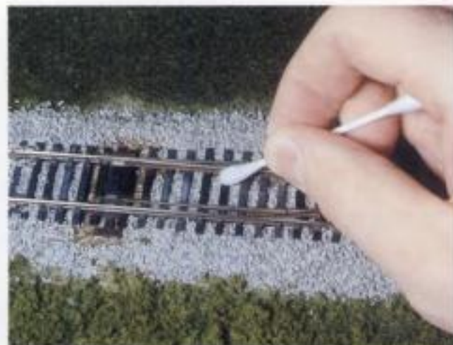
Fig. 12-22. Use a damp cotton swab to soak up glue from the ties under the turnout points.
