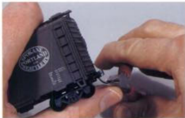
Fig. 3-16. Special pliers for adjusting uncoupling pins are made by Kadee and Micro-Mark, but standard pliers can also be used.
