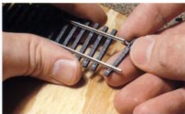
Fig. 9-15. Cut the tie strip under the rail and remove the end tie before laying flextrack.
