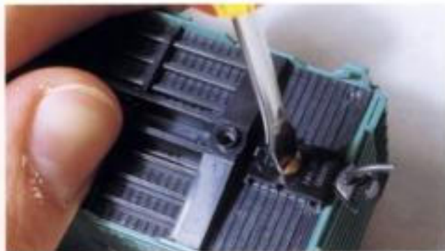
Fig. 3-21. Screw the new coupler and box into place.
