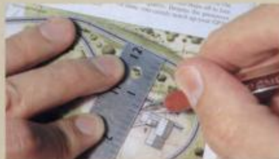
Fig. 2. Measure to find the center point of each curve, then mark it on the track plan.
