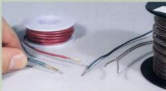
Fig. 1. A sampling of available wire: 14-gauge solid, 18-gauge stranded, 22-gauge solid, and two-conductor 24-gauge solid (speaker wire).
