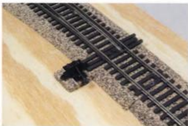
Fig. 9-25. The throw mechanism on this Caboose Industries ground throw connects to the turnout throw bar.
