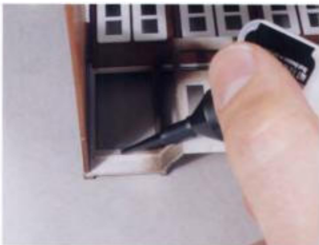
Fig. 11-9. Place clear parts glue sparingly on the inner wall around the windows, then add the clear plastic window glazing.
