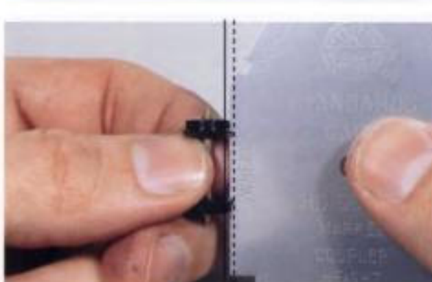
Fig. 4-3. This Athearn wheelset is in gauge, with flanges at the proper depth.
