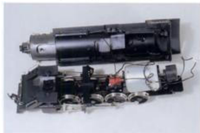
Fig. 5-6. Removing the shell shows the motor (with a small flywheel that protrudes into the cab) and worm, which drives a gear on the third set of drivers.
