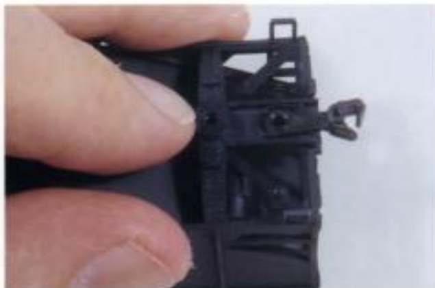
Fig. 3-3. Accurail's Accumate is a two-piece coupler molded in acetal plastic, with a separate steel uncoupling pin (omitted in this view).
