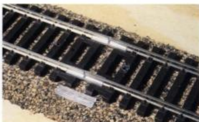
Fig. 9-13. Insulated rail joiners are the easiest way to divide a layout into electrical blocks.
