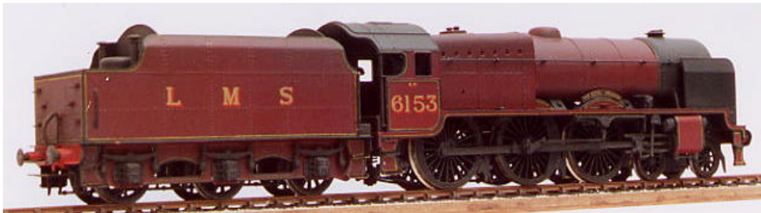
LCP1 (with a TK1) Seen here with a Mainline Royal Scot body. TK1 is a Stanier 4000 gallon riveted tender
