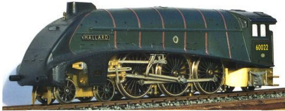
LCP30 Gresley A1/A3/A4 Seen here under a Hornby A4 body.
