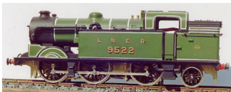
LCP34 N2 0-6-2T, seen with a Dapol plastic body.
