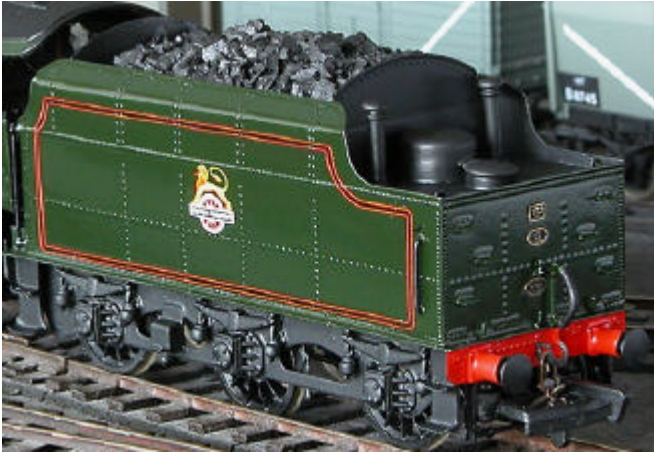
TK1 Stanier 4000 gallon riveted tender. Built and photographed by John Cooper-Smith, who fitted non standard axleboxes for his model of 46202
