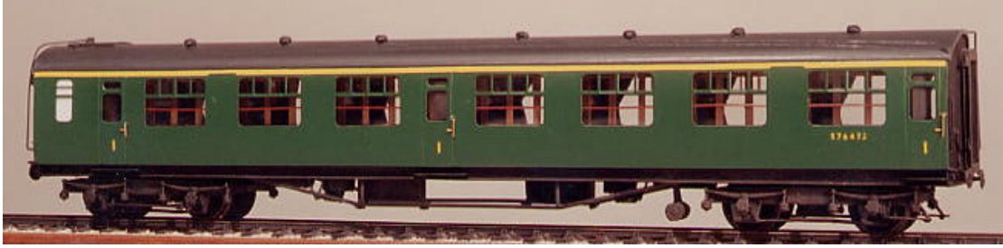
S8 64'6" Semi-Open Brake Third Shallow vents D2123 1946
