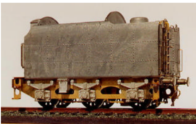
TK14 BR1F, 5625 gallons, 7 tons. Fitted to Southern Region allocated 73xxx and Eastern Region 9Fs
