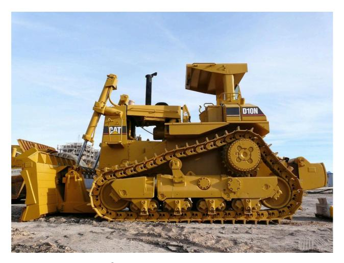
First released in 1987, the Cat<sup>®</sup> D10N Dozer featured an extended track frame for improved traction and stability over the D9L as well as a flywheel horsepower increase on the Cat<sup>®</sup> 3412 diesel engine from 460 HP to 520 HP.
