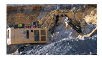
The current lineup of Cat® Next Generation Hydraulic Shovels feature Hydraulic Optimization which dynagroups of pumps, to deliver the exact flow and pressure that each hydraulic function requires. Other converges at maximum flow and pressure regardless of the demand from individual circuits. This new system Shovels up to 15% more fuel efficient, reduces excess heat, conserves energy, and prolongs component life.
