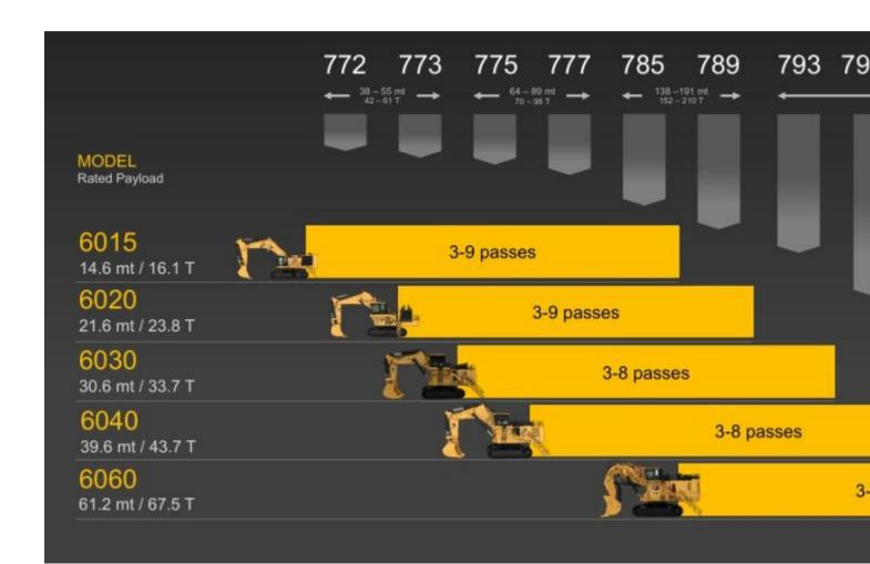
Pass matching and choosing the right Cat® Hydraulic Shovel to compliment a truck fleet has a major important gives a good example of passes required to optimize truck loading and lower cost per ton.
