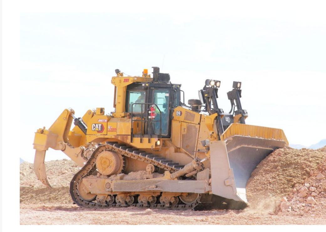
Nearly half of the large dozers Caterpillar® sells are D9 Dozers – and for good reason. They're the smart choice for dozens of applications a environments thanks to unmatched reliability, long life and a wide range of application-specific blades. When equipped with a Universal blather machine has a blade capacity of up to 21.7 cubic yards (17.8 cubic yards with Semi-Universal). Single shank, multi-shank, or winches can be mounted to the rear depending on application needs.
