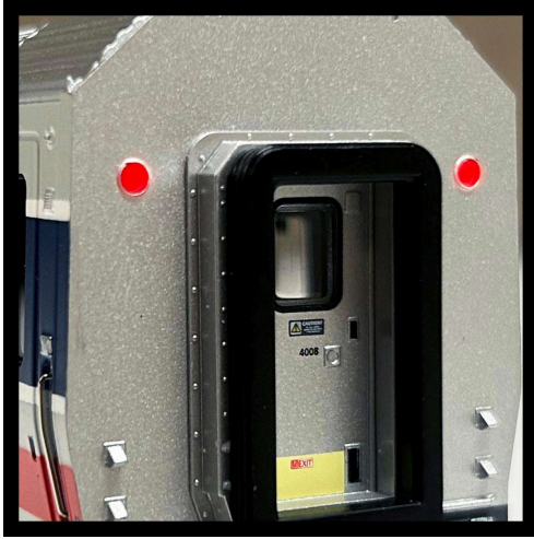
Functioning Controllable Marker Lights
