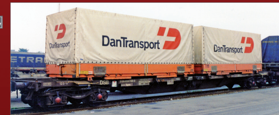
Carro Sgns danese caricato con due casse mobili telonate "DanTransport". DSB Sgns container vogn belæsset med to "DanTransport" veksellad. Danish type Sgns container wagon loaded with two "DanTransport" swap bodies.
