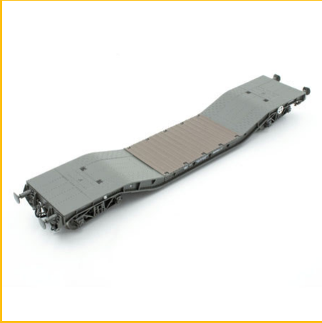
50t 'Warwell' military flat with diamond frame bogies in WD livery (LMS variant) - No.57
