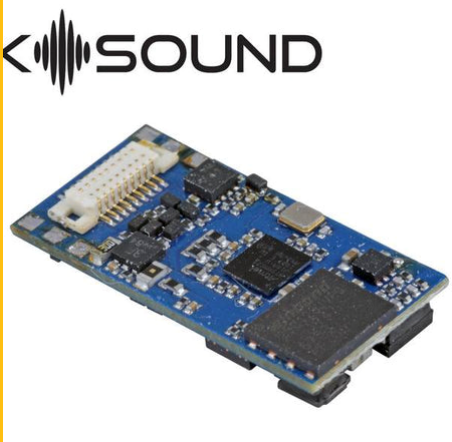
Accurathrash GWR 'Manor' Loksound DCC Sound Decoder
